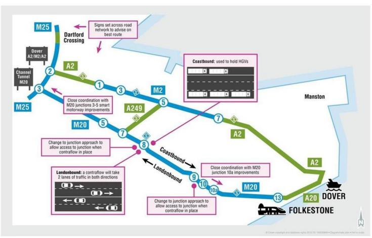
**How It Works -** Coastbound carriageway of M20 between J8 & J9 available to port-bound freight only. London bound carriageway between J8 and J9 to be used in both directions by all other traffic. **Holding Capacity -** Approx. 2,000 HGVs.
